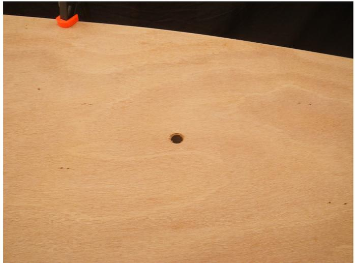
Fit a 1/2" (12mm) flush-trim bit into your router and excavate the slot, starting with the hole you drilled previously.
