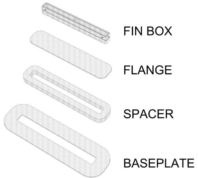
Mix up a 2oz (30ml) batch of epoxy, thickened to paste consistency with Cell-O-Fill, and brush a generous slather onto the the mating face of the spacer.
