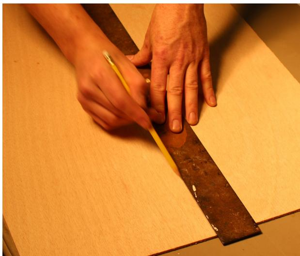
For optimal performance, the fin box should be positioned so that the **back edge** of the opening is 7-1/2" (190mm) forward of the transom, or "tailblock" in paddleboard lingo.
