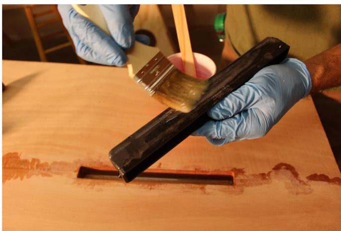
Press the fin box into the slot...
