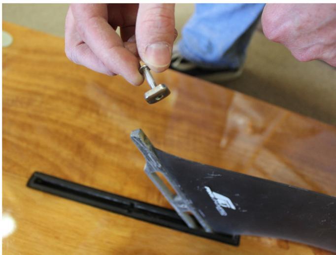
Slide the nut into the groove...
