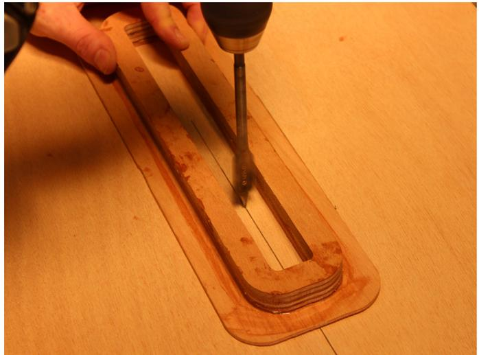
Flip your paddleboard upside down onto your sawhorses. Here's the hole you just drilled from the underside of the board.
