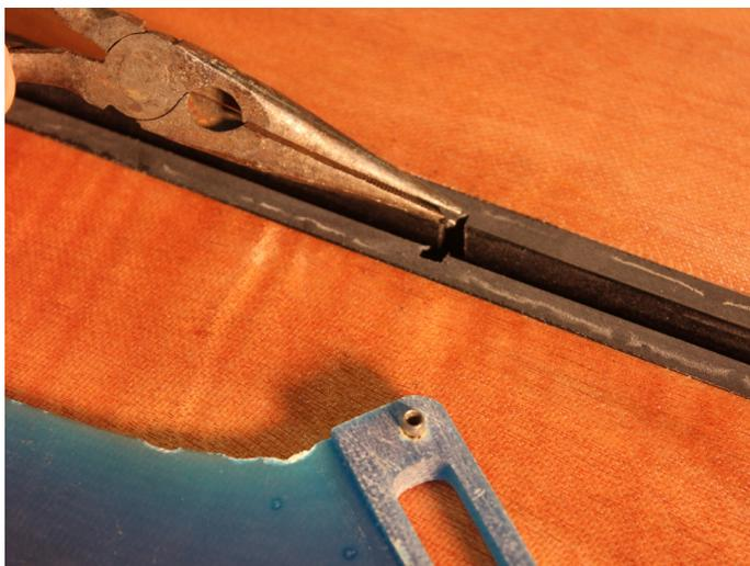
Time to test-fit your fin! The fin pin drops into the center slot, then slides forward or aft along the internal track.
