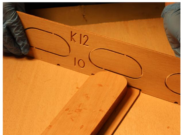
Here's how your frames should look once they have been notched to accept the fin box. Frame 11 for the Kaholo 14 is shown on the left, frame 10 for the Kaholo 12-6 on the right.
