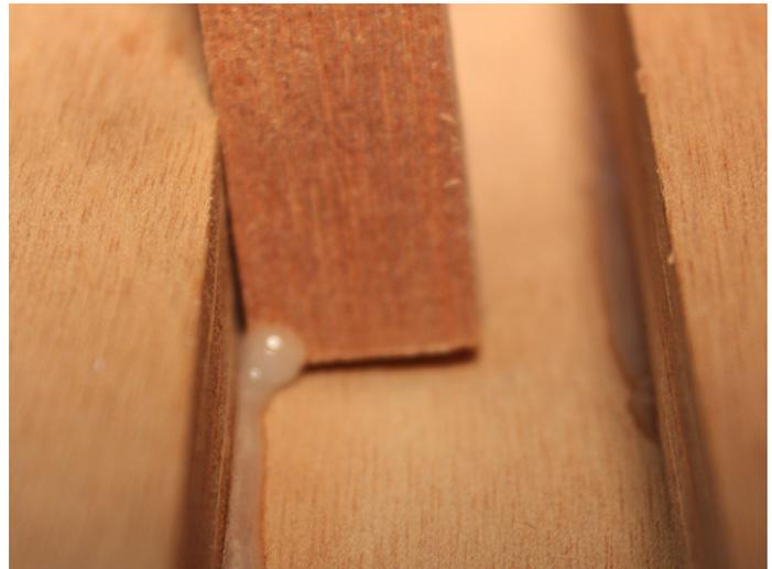
Once the epoxy has cured, test-fit the plastic fin box into the slot. The small tabs on the fin box will set the depth; do **not** sand these off! The fin box itself should protrude approximately 1/4" (6mm) from the bottom of the board.
