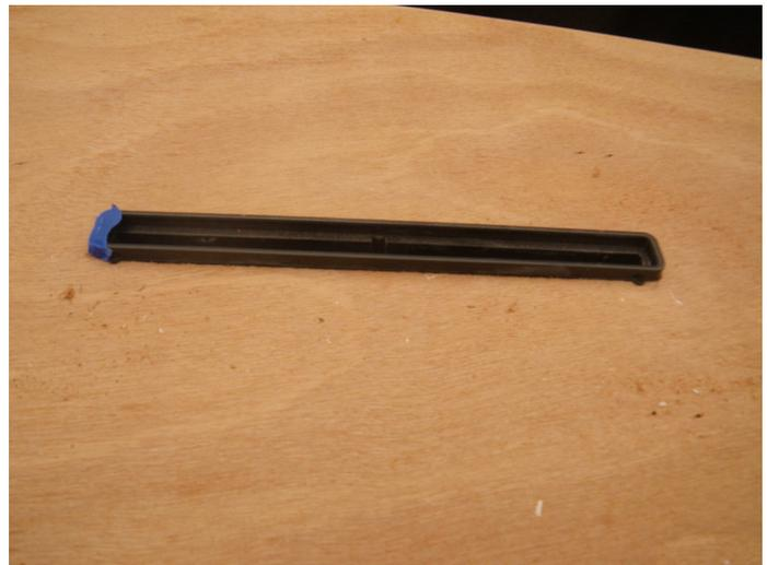
If you are struggling to get the fin box to fit, check the slot to make sure there are no drips of epoxy preventing you from inserting the box. If the inside of the slot is smooth, lightly sand the exterior of the fin box until it slips neatly into the slot.
