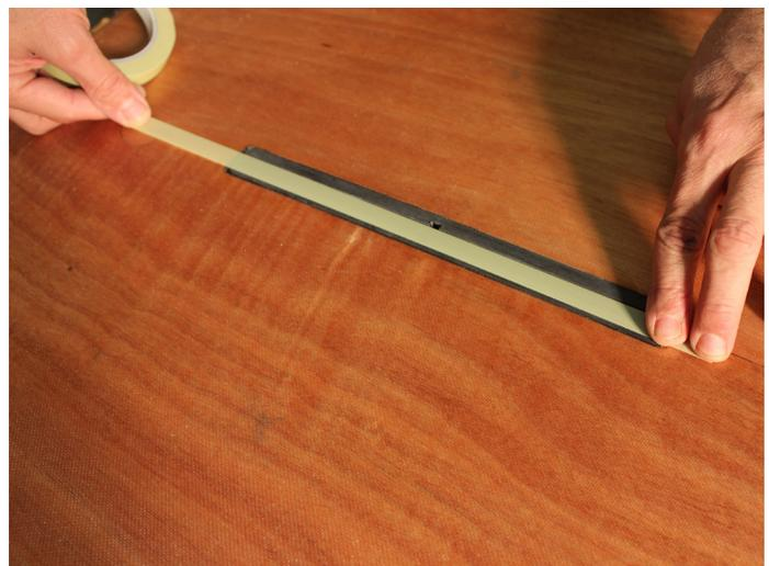
Here, we're varnishing the bottom of the paddleboard, right over the taped-off fin box. At this point, you will have removed the first batch of tape when you cut the fiberglass around the fin box. You will need to re-apply fresh tape before varnishing or painting.
