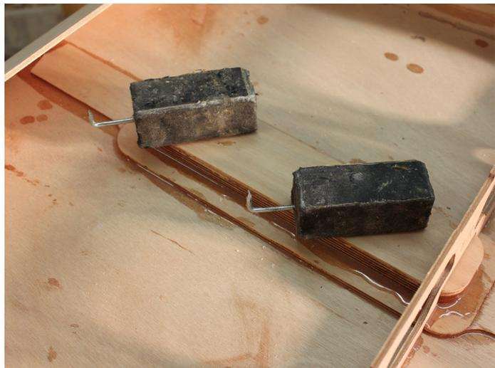
...but before the epoxy hardens, crawl under the paddleboard and scrape out any excess epoxy that may have squeezed out from the cap.
