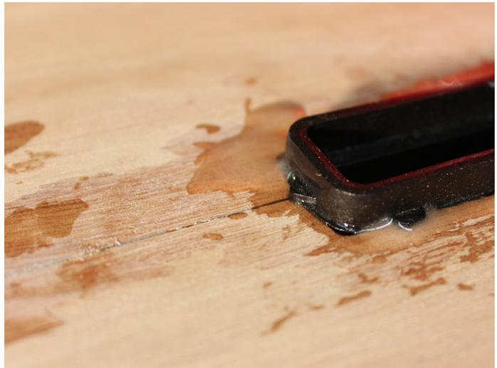
Once the epoxy has fully cured, trim the excess fin box material with a sharp block plane...
