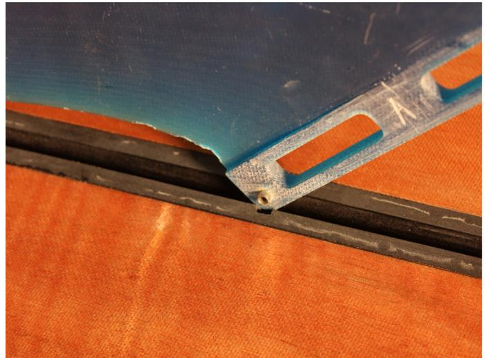
If the fin is too wide to fit into the box, lightly sand the inside faces of the fin box until the fin can be fully inserted.
