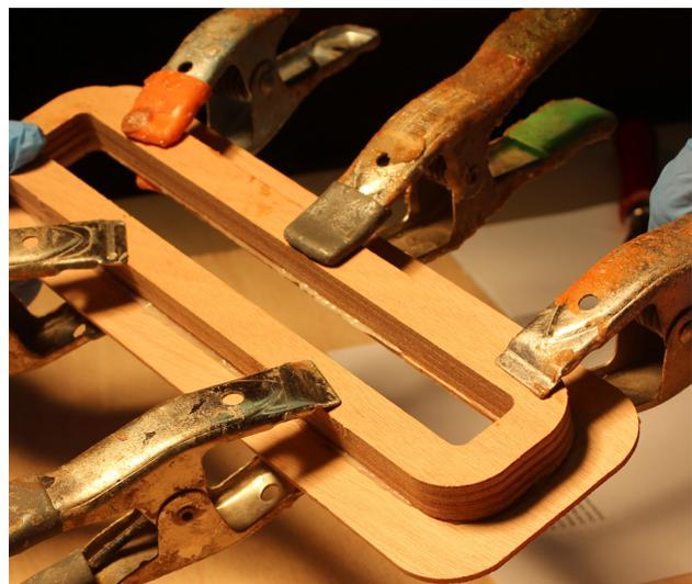
You'll know that you have used enough epoxy if it squeezes out from between the two parts. Carefully scrape off the excess goo and set aside the assembly. Allow the epoxy to cure for 24 hours before removing the clamps.
