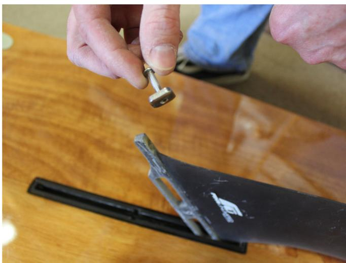
Slide the nut into the groove...
