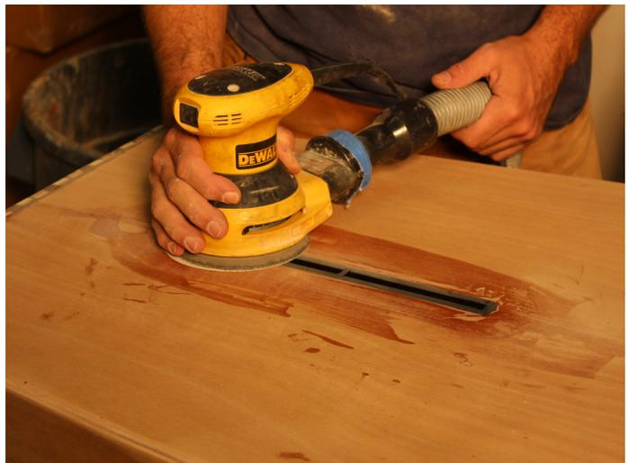
The fin box should be perfectly flush with the surrounding plywood bottom panel.
