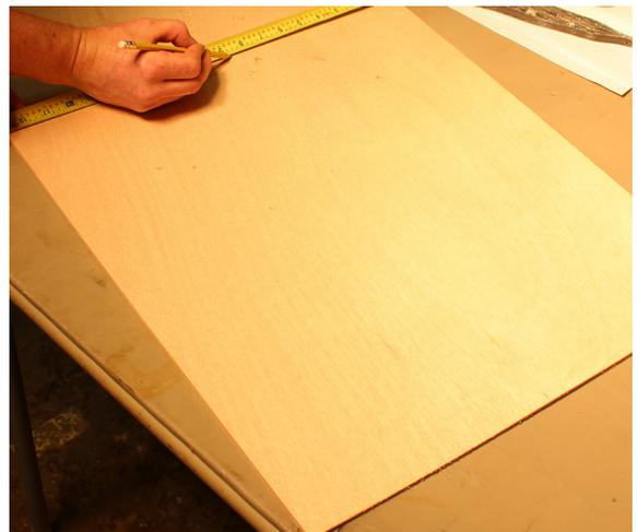
Take two transverse (widthwise) measurements along the back of the aft bottom panel, one measurement at the back edge (*above, left*), and another about 12" (300mm) forward (*above, right*). Mark the centers.
