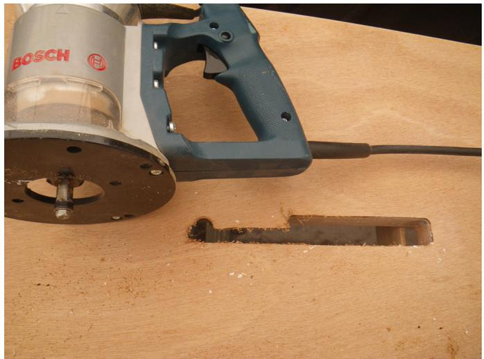
Here's the finished slot, perfectly cut by the router.
